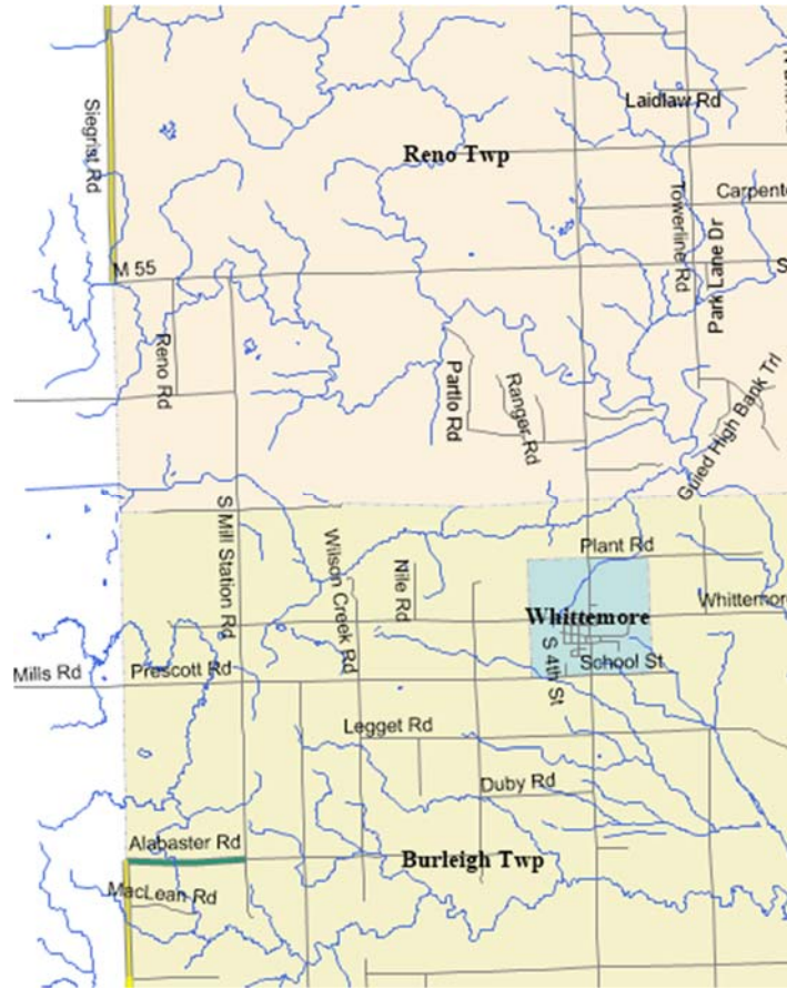
Figure 25: Map of the current IBR for surface width with good (22' and greater) shown in green, fair (16' to 21') shown in yellow, and poor (15' or less) shown in red. Only Primary unpaved roads owned by ICRC are shown.
