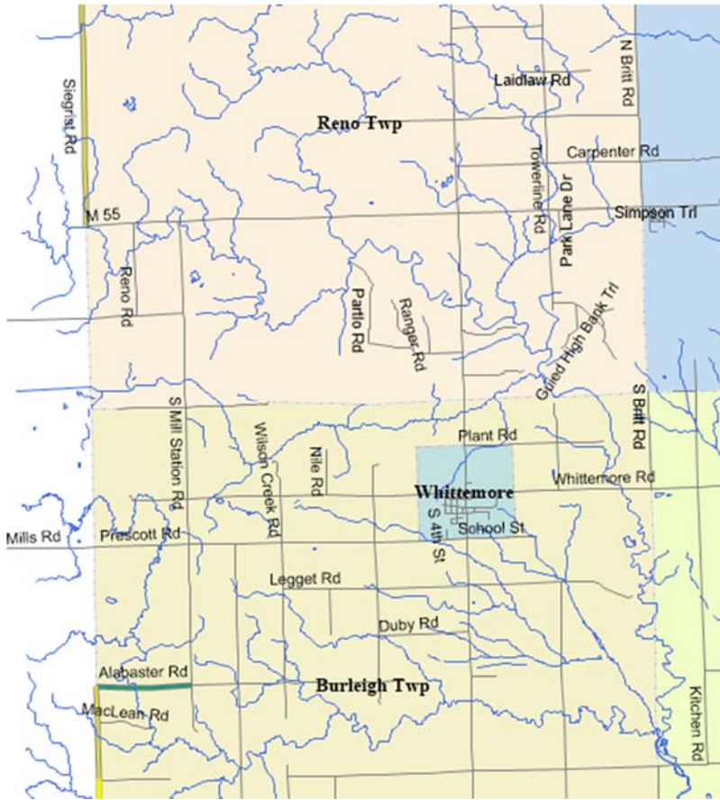
Figure 26: Map of the current IBR for drainage adequacy with good (2' or more) shown in green, fair (0.5' to less than 2') shown in yellow, and poor (less than 0.5') shown in red. Only Primary unpaved roads owned by ICRC are shown.
